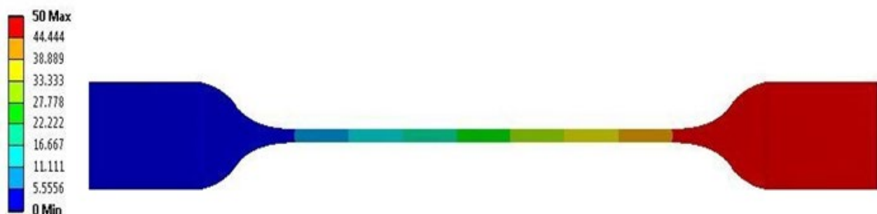
Fig. 4. Deformation state of uniaxial tensile finite element model
